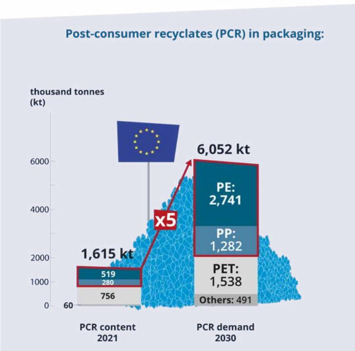
Source: Material flow diagram 2021, Conversio. PCR demand in 2030 is based on an IC estimate for Germany. Simplifying assumptions: 50 % of the processing volumes are contact-sensitive packaging and no company uses more than is legally required by quotas.
